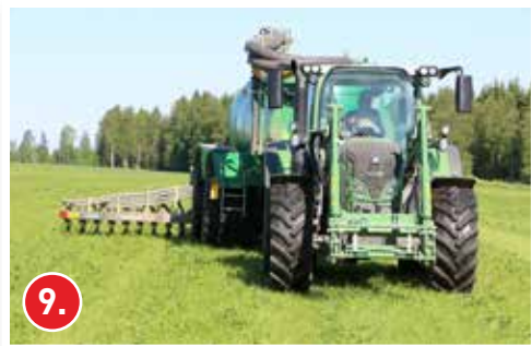
With crab steering, the tractor and slurry tanker can travel along different tracks in the field, thus considerably reducing soil poaching.
