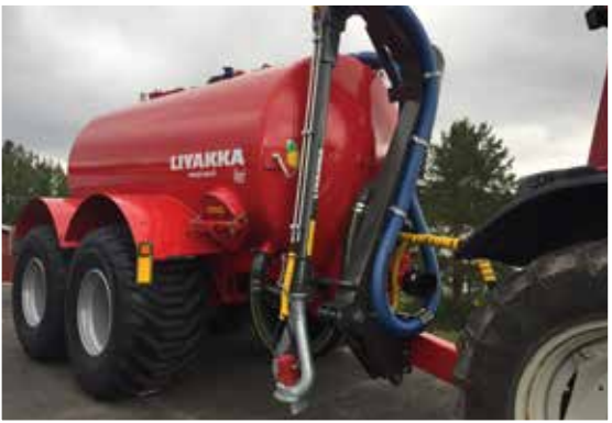
5" front-mounted pump crane
