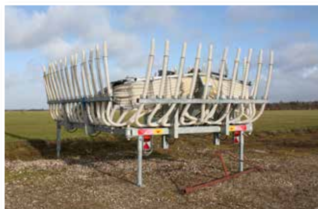
12 m and 16 m drip hose boom with retractable hoses
