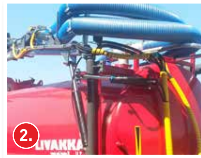
Side-mounted pump crane 6"
