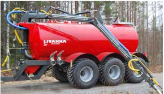
8" centre-mounted pump crane
