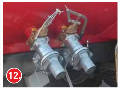
Bottom fill with foam connection. 6" pipes.
