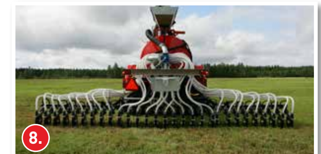
LHDD hydraulic double disc injectors
