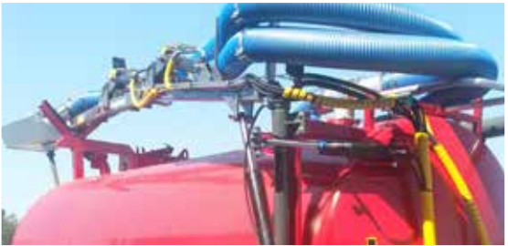
6" side-mounted pump crane
